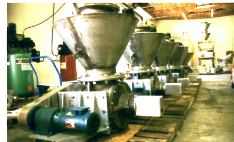
FINISHED CDC AIRLOCKS & VENT HOPPERS READY FOR SHIPPING
